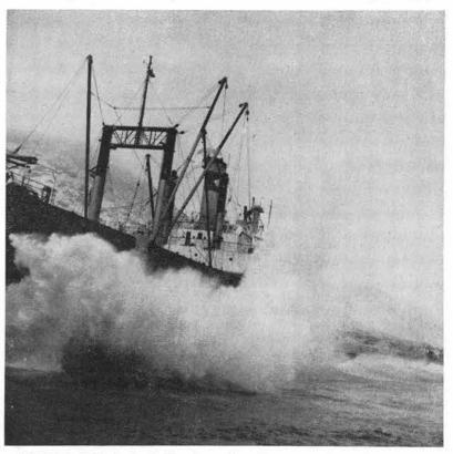
WRECKED SHIP looked like this when the ground swells struck it broadside, pouring water into the holds and causing the entire ship to shake. The ship lists four degrees toward the sea, and is settling.
